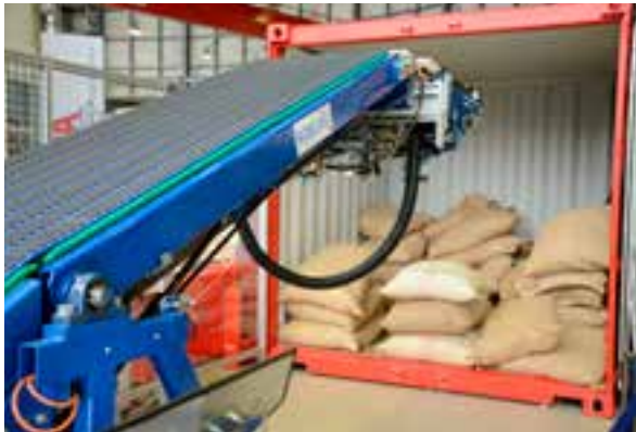
Der RobLog-Industrial-Demonstrator im BIBA entlädt Kaffeesäcke. Rechts: Der Greifer. (Fotos: David Schumacher) | The BIBA's RobLog Industrial Demonstrator unloads coffee sacks. On the right side: The gripper (Images: David Schumacher)
