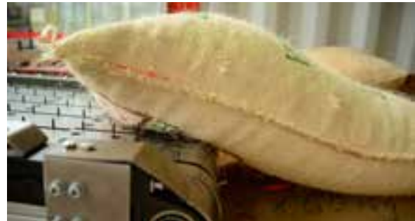
Der RobLog-Industrial-Demonstrator im BIBA entlädt Kaffeesäcke. Rechts: Der Greifer. (Fotos: David Schumacher) | The BIBA's RobLog Industrial Demonstrator unloads coffee sacks. On the right side: The gripper (Images: David Schumacher)
