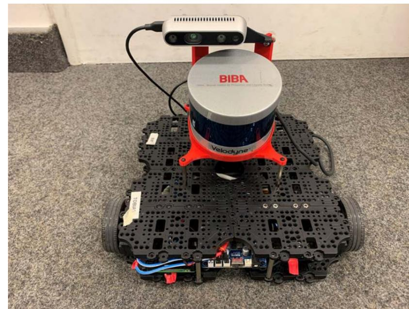
In the **Development of a navigation system for AGVs based on optical markers** project, bachelor's students on the Systems Engineering degree programme have developed an autonomous vehicle system that can orientate itself in space using optical markers and navigate within it. One area of focus was on the development and optimisation of software and algorithms for the stable detection and localisation of route markers and POIs as well as the resulting implications with regard to route planning.
