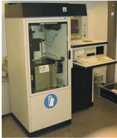
Anfänge des 3D-Drucks: Eine der ersten Stereolithographie-Anlagen Europas stand im BIBA. (Bild: BIBA) | The beginnings of 3D printing: One of the first stereolithography systems in Europe was located at BIBA. (Image: BIBA)
