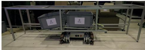
Left: Prototypical automated guided vehicle with mecanum chain drive | Above: AGV with KLT transfer station in pilot test, Photos: BIBA
