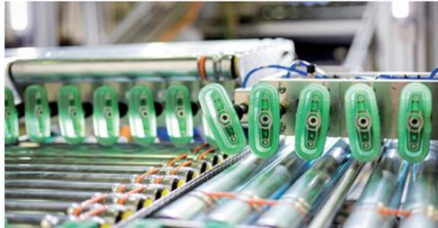
Left: IRiS-Container Unloading System, Source: BIBA | Above: Vacuum-based gripping shovel with integrated conveyor system, Photo: Jan Meier
