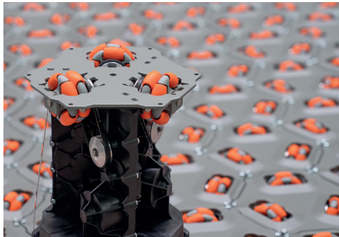
Left: Individual cell of the celluveyor, removed from the system | Above: Celluveyor in use for sorting parcels, Sources: cellumation GmbH
