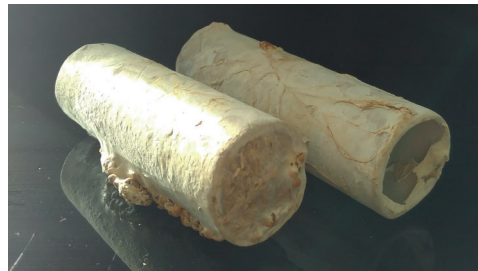
Left: Paper cylinder overgrown with the mycelium of the tinder fungus ( Fomes fomentarius ) | Above: Hollow cardboard cylinder with and without straw substrate filling, overgrown with mycelium of the oyster mushroom ( Pleurotus Ostreatus ), Sources: Armin Schmid
