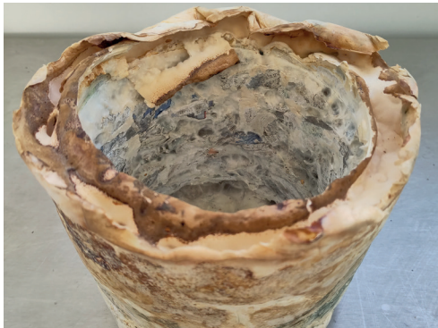
Left: Paper cylinder overgrown with the mycelium of the tinder fungus ( Fomes fomentarius ) | Above: Hollow cardboard cylinder with and without straw substrate filling, overgrown with mycelium of the oyster mushroom ( Pleurotus Ostreatus ), Sources: Armin Schmid
