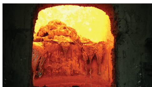
Left: Planned control of the aluminium melting furnace | Above: View of the melting bridge through the maintenance, Sources: ZPF
