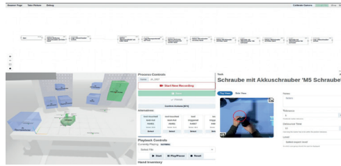
Left: Projection of a graphical user interface onto the workspace using a projector | Above: User interface for an assembly planner including the digital twin of the workplace, the assembly instructions, and the generated assembly process, Sources: BIBA GmbH
