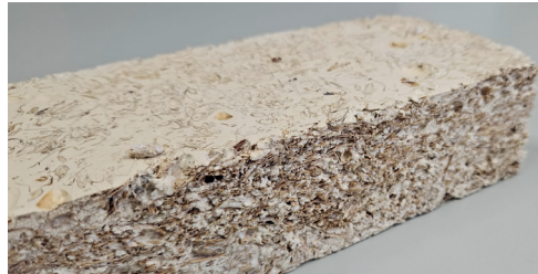
Left: Mycelium of the fungus Ganoderma resinaceum , Image: (Binocular) Uni Göttingen/Michael Unger | Above: Mycelium-based composite material made from straw, husks and starch, Image: Uni Göttingen/Michael Unger
