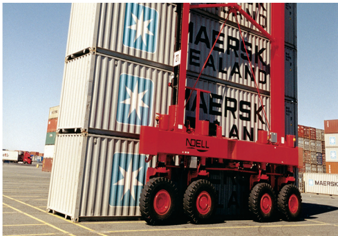
Left: Straddle Carrier in action, Source: bremenports GmbH & Co. KG Above: Handling of a ship in the container terminal, Source: EURO-GATE GmbH & Co. KGaA, KG
