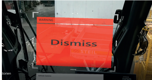
Left: Setting down a load precisely without visual contact, Photo: Steil Kranarbeiten GmbH & Co. KG | Above: superimposing a warning message in the field of view with AR data glasses, Photo: BIBA
