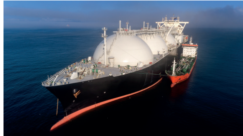
Left: Representation of cold sections of a pipe system compared to the environment and detected leaks | Above: Bunkering of a LNG carrier, Photo: © vladsv/Fotolia.com
