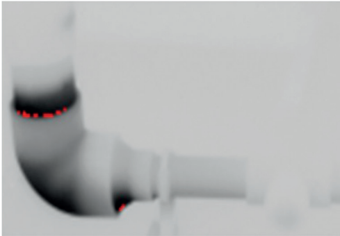
Left: Representation of cold sections of a pipe system compared to the environment and detected leaks | Above: Bunkering of a LNG carrier, Photo: © vladsv/Fotolia.com
