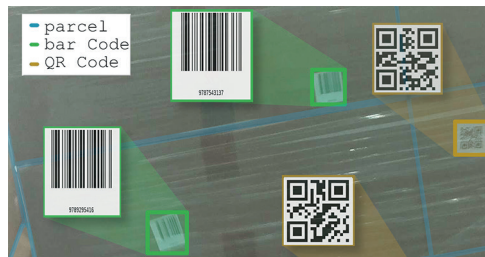
Left: Schematic of the DroneStock solution | Above: Using AI-based object detection, individual parcels (blue) are detected and relevant bar and QR codes (green and orange) registered, Figures: Benjamin Staar
